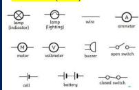
Circuits can be represented as diagrams using symbols for each component
